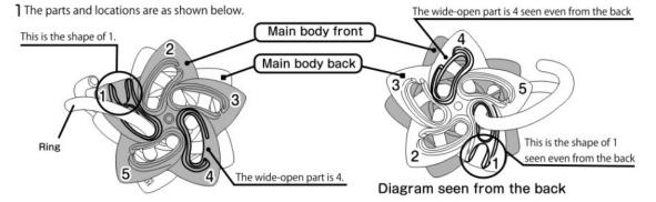
2 Moving the back and front of the main body left and right to misalign them will create a gap large enough for the ring to pass through the part overlapping the main body. Rotating the ring while passing it through the gap enables the ring to be moved to various positions.
