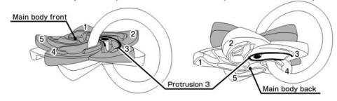
5 Rotate the back of the main body clockwise. Simultaneously, move the ring to the back and cause the ring to tilt.
