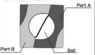
2 Keep Part A and lower ball half from moving, then twist the Part B and upper ball half together.
